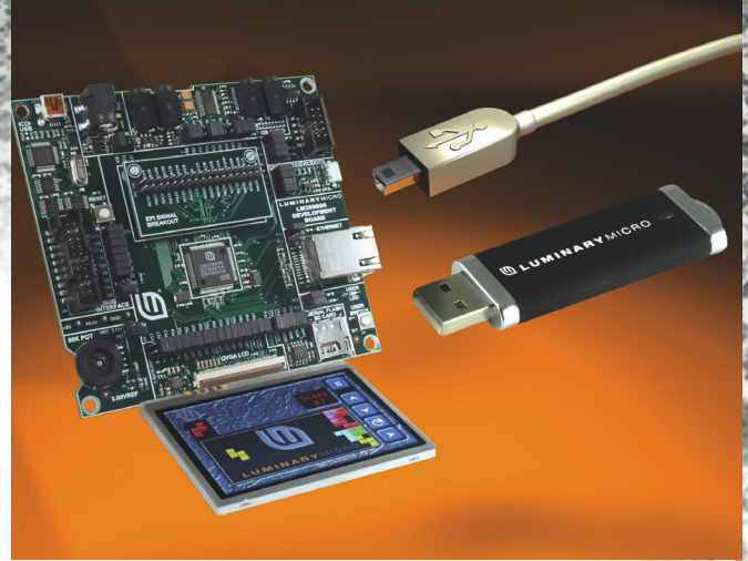
Figure 4 The DK-LM3S9B96 development kit supported the port to Texas Instruments' ARM Cortex-M3 processor.
